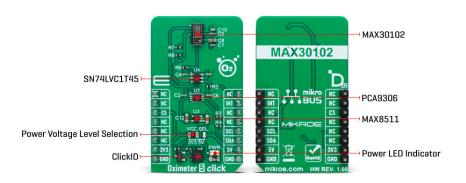
The SpO2 subsystem of the MAX30102 contains ambient light cancellation (ALC), a continuoustime oversampling sigma-delta ADC with 18-bit resolution, and a proprietary discrete-time filter. The ALC has an internal Track/Hold circuit to cancel ambient light and increase the effective dynamic range. The MAX30102 also has an on-chip temperature sensor with an inherent resolution of 0.0625°C for calibrating the temperature dependence of the SpO2 subsystem.
