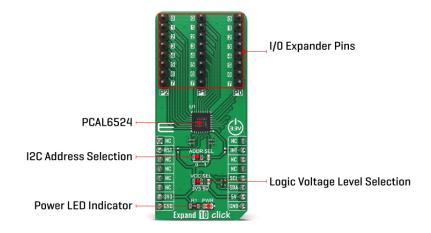
The PCAL6524 implements Agile I/O features specifically designed to enhance the I/O. These additional features are programmable output drive strength, latchable inputs, programmable pull-up/pull-down resistors, maskable interrupt, interrupt status register, programmable opendrain or push-pull outputs.
