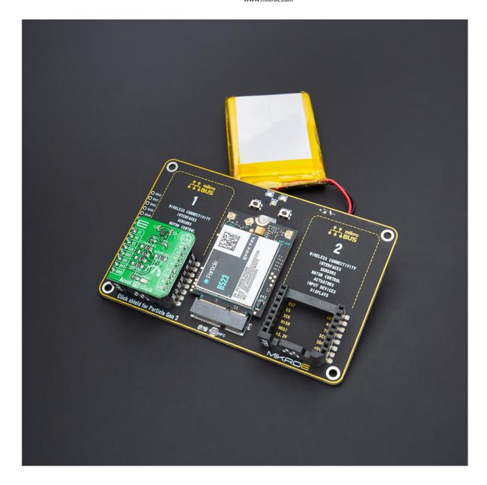
When the battery is connected to the battery connector on the bottom side of the board the power will be provided to the Click Shield from it, including mikroBUS™ sockets.
