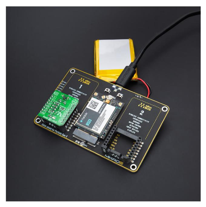
When the USB type C connector and the battery is connected to the Click shield for Particle Gen 3 at the same time, the mikroBUS<sup>m</sup> sockets will be powered from the USB Type C connector.
