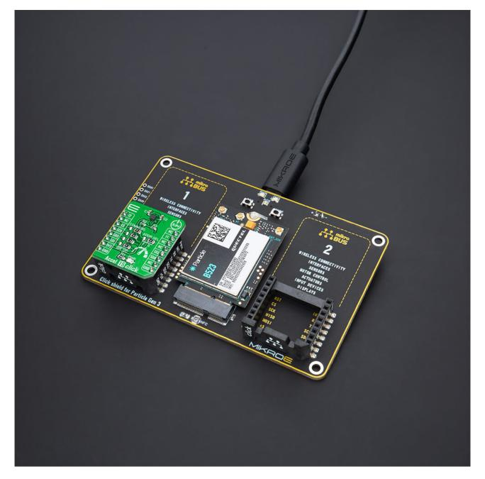
When the USB type C connector is connected to the Click shield for Particle Gen 3, the connected Click shield and mikroBUS™ sockets will be powered from it.
