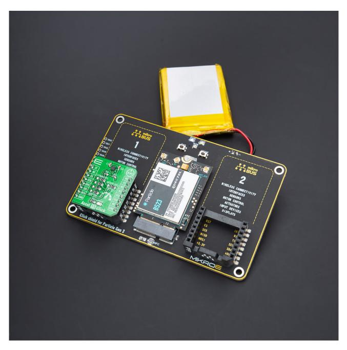
When the battery is connected to the battery connector on the bottom side of the board the power will be provided to the Click Shield from it, including mikroBUS<sup>™</sup> sockets.
