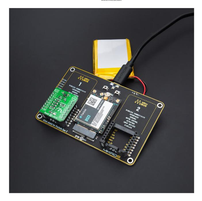
When the USB type C connector and the battery is connected to the Click shield for Particle Gen 3 at the same time, the mikroBUS $^{\text{m}}$  sockets will be powered from the USB Type C connector.
