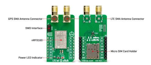
The nRF9160 is specifically designed to take full advantage of the energy efficiency associated with the LTE-M and NB-IoT standards. It supports both the PSM and eDRX power-saving modes, enabling the nRF9160 to sleep for a longer period. At the left side of this Click board<sup>™</sup>, there is an additional header, labeled as SWD, which offers full support of debugging and programming capabilities through the serial wire debug (SWD) interface (SWDIO, SWCLK, and SWO).
