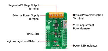
The output voltage of the TPS61391 is externally adjustable using a resistor divider network. The relationship between the output voltage and the resistor divider is given by the equation:
