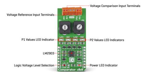
Comparator Click communicates with the host microcontroller with each output using its own interrupt pin on the mikroBUS™ socket labeled O1 and O2. In addition, every independent output has its own red HIGH and green LOW LEDs for visual presentation, labeled LO1, HI1, LO2, and HI2.
