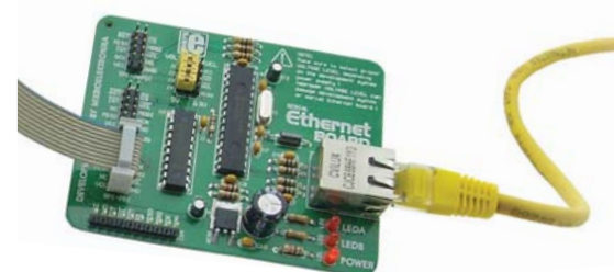
Figure 1. MikroElektronika's Serial Ethernet module with ENC28J60 chip
