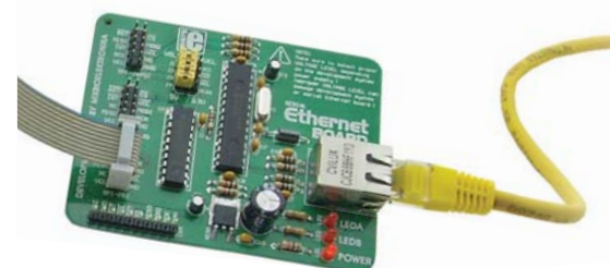
Figure 1. MikroElektronika's Serial Ethernet module with ENC28J60 chip
