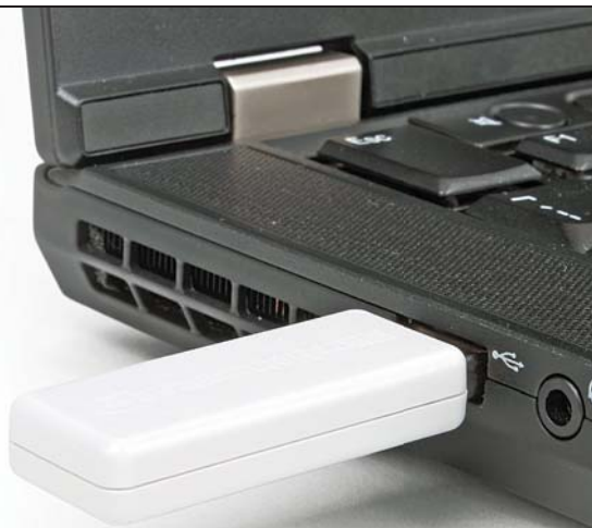
Figure 1-3: USB Dongle plugged into Laptop USB host connector
